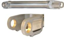
Full size landing gear side stay for Airbus A320. 35% lighter than aluminium standard part. Net shape manufacture of tube and clevises to avoid welds.
