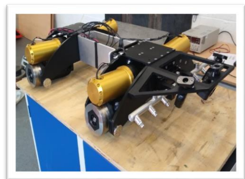
Figure 1: iFROG robot – Robot 1 (cleaning and corrosion mapper)
